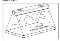
Figure 2. Area of optimum charge neutralisation for 92260
