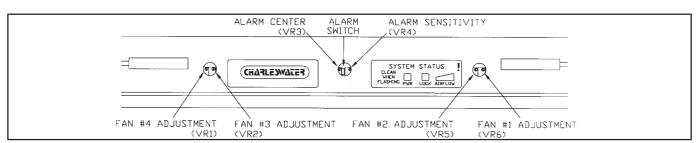
Figure 6. Calibrating C/E Ioniser
