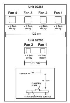
Figure 7. Balance under < 10 volts. When set under lab conditions, 5 volts is attainable.
