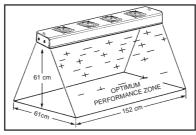
Figure 3. Area of optimum charge neutralisation for 92261
