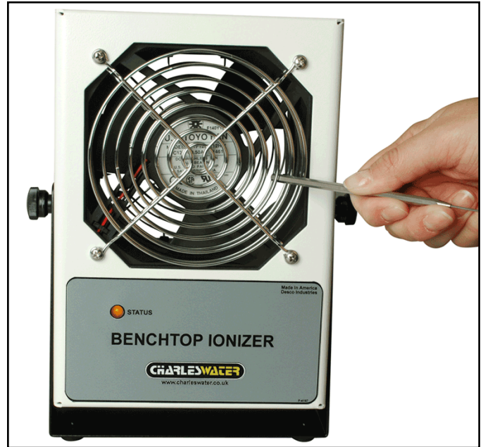
Figure 6. Shorting the ioniser's fan grills with a metal probe to test the alarm
