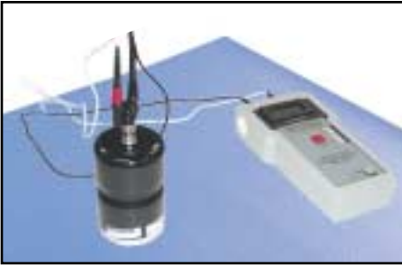
Figure 2. Concentric Ring Probe connected to Surface Resistance Test Kit
