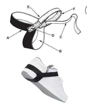
"Highly mobile personnel are almost impossible to ground with a wrist strap. In these cases an alternative grounding method may be necessary in combination with wrist straps.
