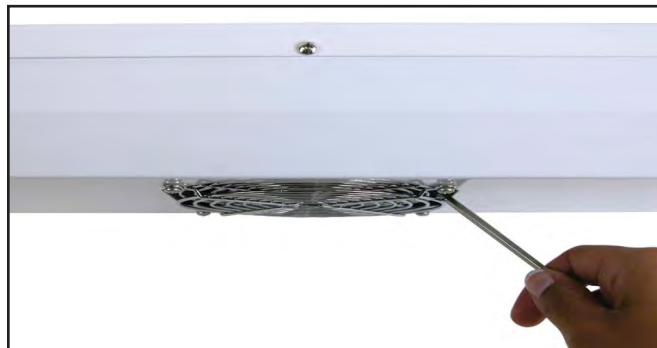
Figure 6. Shorting the ionizer's three fan grills
